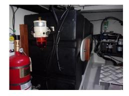
The rubber piping was all found to be in a good condition, the correct ISO standard, and secured properly to the boat. The fuel filters were both found to be in a good condition. No evidence of any diesel bug or water contamination in either of the fuel filters was noted. All metal fittings have been earthed correctly.
