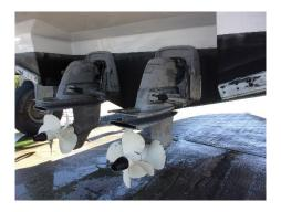
Both transom shields were found to be in a good condition, with no evidence of damage or corrosion noted during the survey
