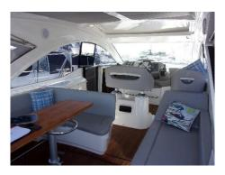
The cockpit gelcoat was found to be in a good condition, with no areas of major cosmetic damage noted during the survey
