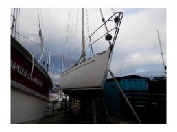
Moisture readings were taken over the entirety of the topsides and were found to average 10 on both sides. These averages are both low and not an issue to the vessel.
