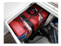
The fuel tank was found to be in a good condition, with no areas of damage noted. The fuel tank is properly secured to the vessel, and cannot move around in the aft locker.
