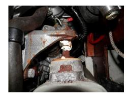
The grease packed stern gland was found to be in a good condition, with no signs of damage noted.
