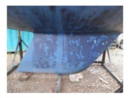
Keel bolts: All keel bolts were found to be in a good condition, with no signs of movement, or "weeping" noted.
