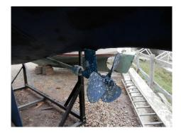
Anodes: There is a shaft anode, and a small "P" bracket circular anode, fitted to Both anodes are depleted, showing that they have been effective this season. Both anodes should be replaced for the next season.
