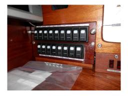
During the survey, every item on the switch board was tested. There were no issues with the switchboard, and everything worked as it should. The masthead navigation light could not be seen working due to the bright conditions.
