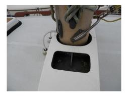
Moisture readings of the area of coachroof surrounding the mast deck plate were taken and found to all be acceptable.
